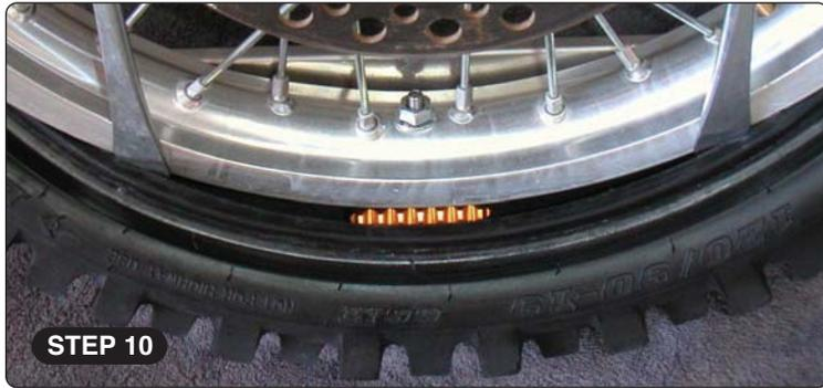
**11** Once the rim is **COMPLETELY** inside the tire, use the tire irons to start pulling the beads back onto the rim. **IMPORTANT:** Always start **opposite** the rim lock and **FINISH pulling the last of the tire bead onto the rim at the rim lock location**. Flip the wheel over and repeat the same procedure again. **FINISH pulling the last of the tire bead onto the rim at the rim lock location**.
